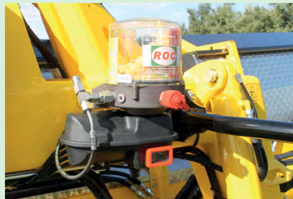
Automatic greasing system optional for all trailed models
