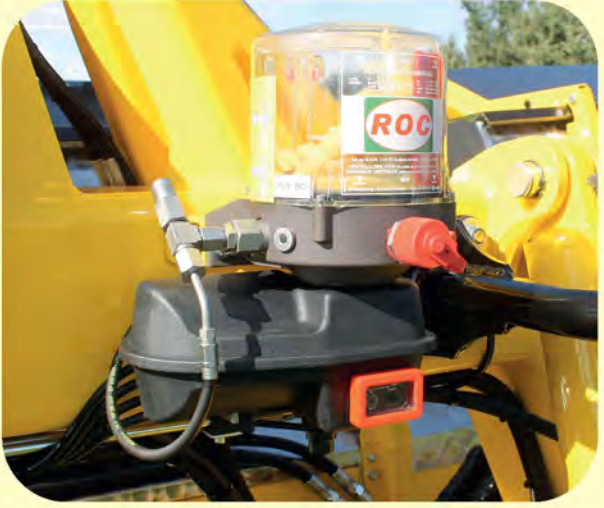
Automatic Grease system
