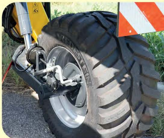
Airbrakes system homologated Mother Reg. Optional for all trailed models
