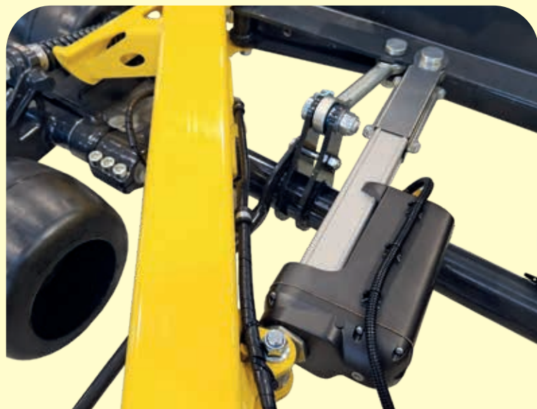
Tandem wheel electrical adjustment Optional for ST 1150 - ST 1000 - ST 920 - ST 870 - ST 730 Standard for ST 380
