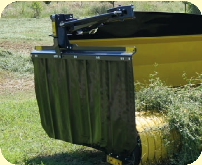
Hydraulic swath guards (right and left side) Optional for RS 1150 - RS 1000 - RS 920 RS 730 - only available right side Manual right swath guard optional for RS 380
