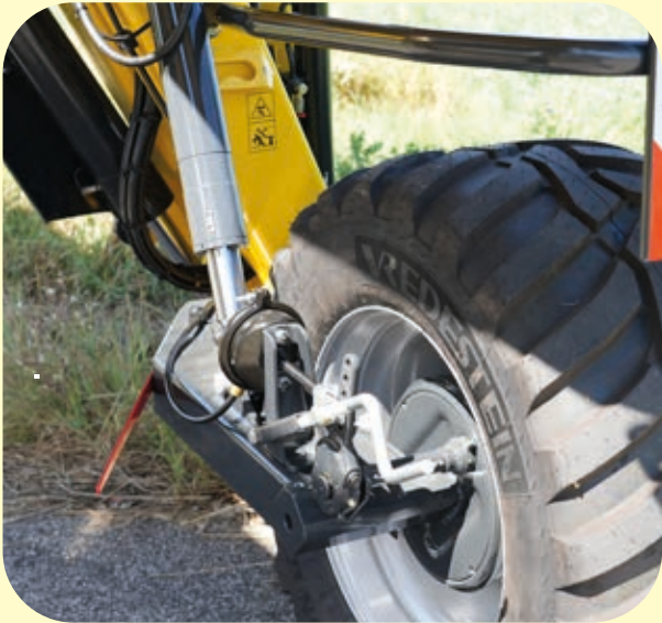
Airbrakes system homologated Mother Reg. Optional for all trailed models
